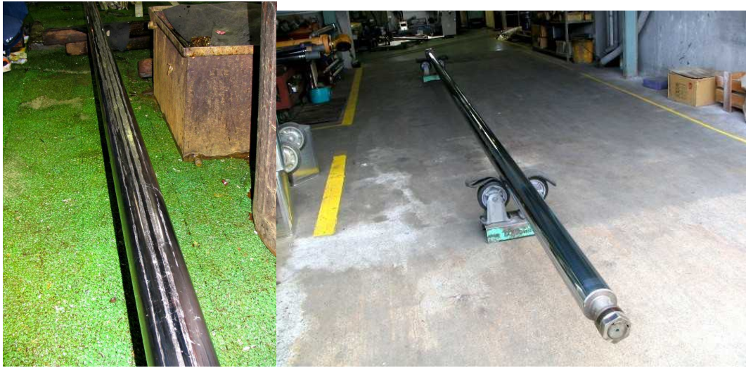
Left: The rod of a Harbor Crane, exceeding 6m in length. Featuring pits, nicks and marks made by foreign substances. Right: After repair, it has been restored with hard chrome plating.
