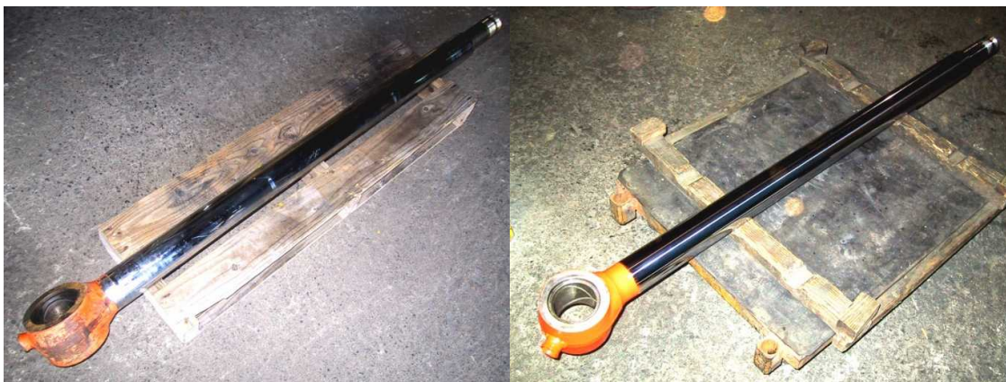
Left: A damaged piston rod from Hitachi Construction Machinery Co., Ltd. Right: After repair; a picture of the same piston rod repaired with hard chrome plating
