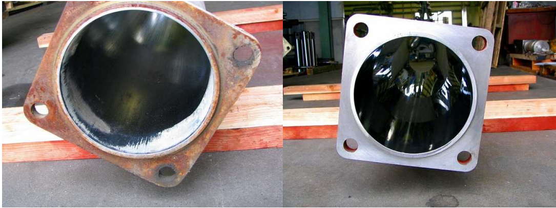
Pictured is the pumping cylinder of a concrete pumping vehicle. Left: Before repair. Right: After repair.
