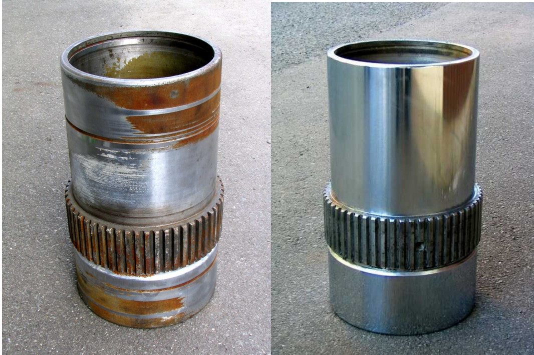
Pictured is the driveline of a concrete pumping vehicle. Left: Before repair. It has been worn out by raw concrete. Right: After repair.
