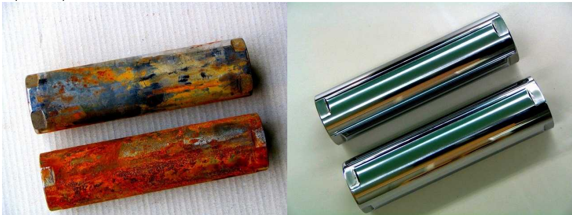
This is an image of a high-pressure chemical injection pump plunger. Note how the item has been corroded by chemicals. Left: Before repair. Right: After repair.
