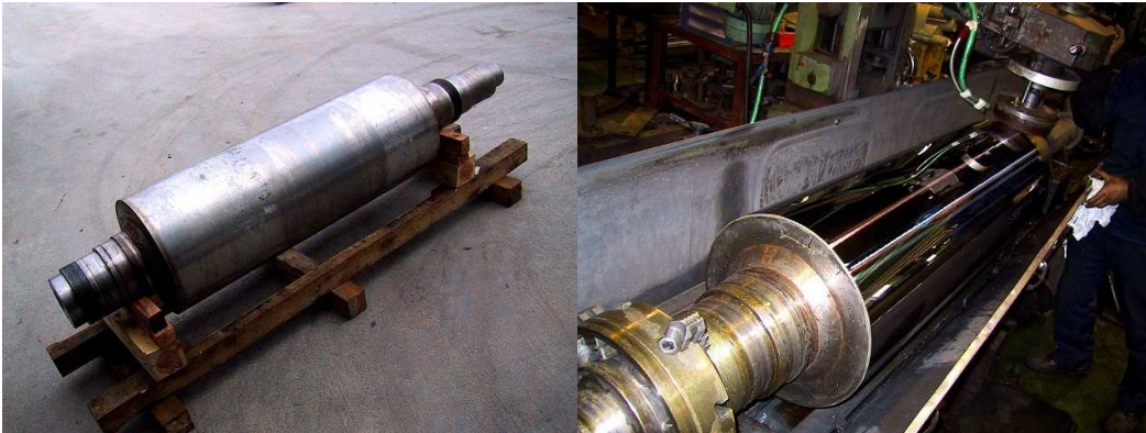
Left: A rolling mill roll used in a steel mill. Numerous surface scratches can be seen. Right: Scratches in the process of being removed through the usage of the chrome plating process.
