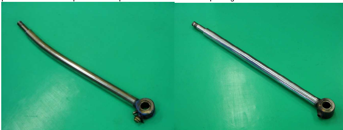
Left: A damaged piston rod from Hitachi Construction Machinery Co., Ltd. Right: After repair; a picture of the same piston rod repaired with hard chrome plating
