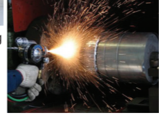
●Wire frame spraying
