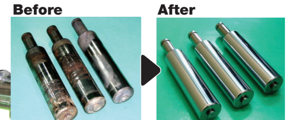
Piston Rod Restoration
